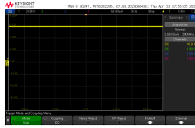
Fig. 6. T3 collector – LED driver transistor switched output.
